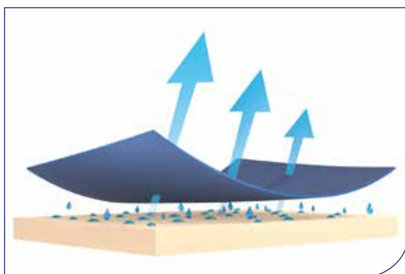
Figure 4. The hydrophobic inner layer pushes moisture onto the outer surface of the garment, while the hydrophilic outer layer pulls any moisture away. This push-pull effect wicks moisture away from the skin
